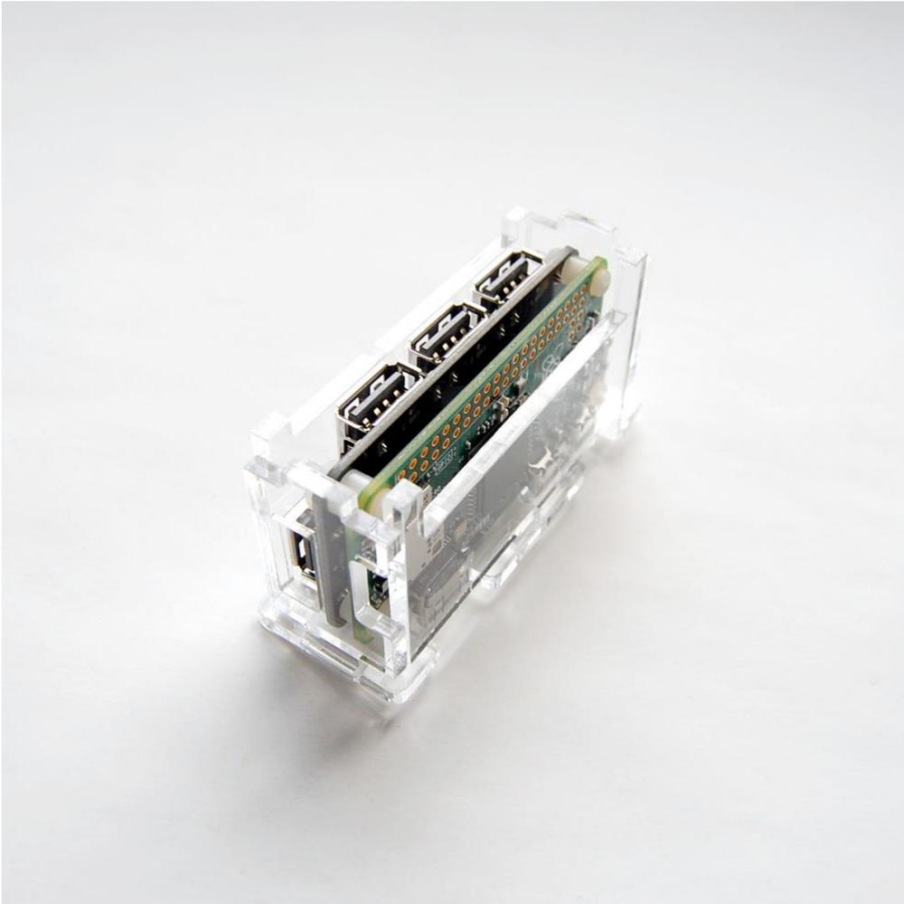
Also pay attention to the other side, for Raspberry Pi Zero V1.3 there is a camera connector, which should be placed in the window:
