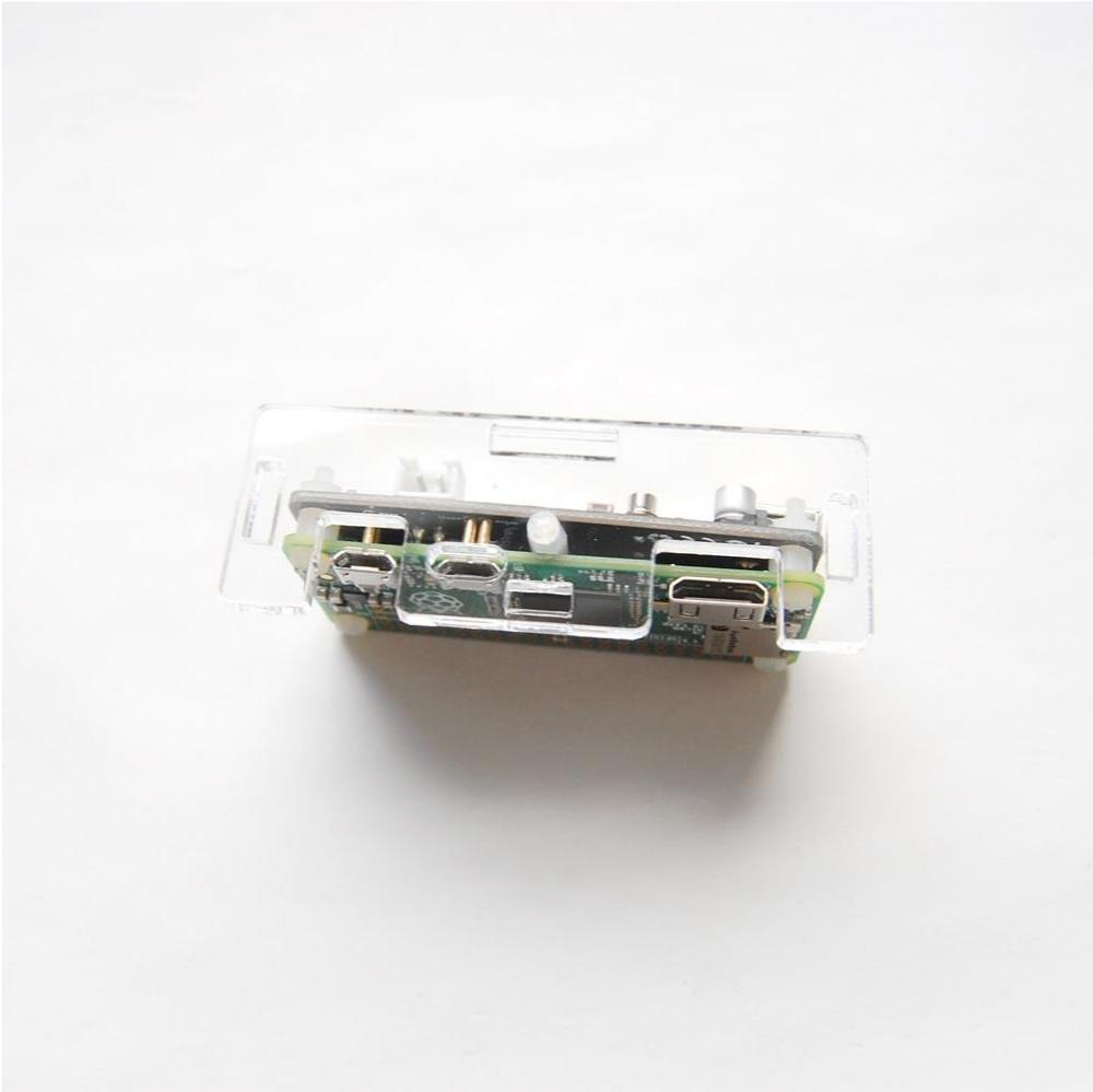
Place it up side down, and put the 4 pieces around your Raspberry Pi Zero and Zero4U. Please pay attention to the sheet that has window for SD card, and make sure it gets placed in correct direction, or the SD card slot could be covered by mistake.
