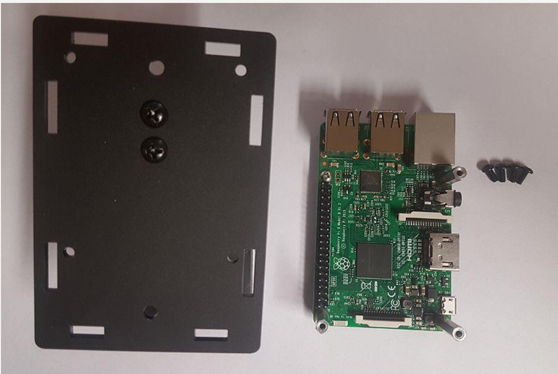
Now we need to attach the Pi to the rear plate using four 1/4" black screws.
