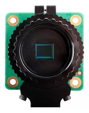
The Raspberry Pi High Quality Camera is the latest camera accessory from Raspberry Pi. It offers higher resolution (12 megapixels, compared to 8 megapixels), and sensitivity (approximately 50% greater area per pixel for improved low-light performance) than the existing Camera Module v2, and is designed to work with interchangeable lenses in both C- and CS-mount form factors. Other lens form factors can be accommodated using third-party lens adapters.
