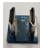
PI3 HDMI PCB Connector (item#7)
